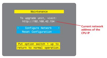
The Maintenance menu should display the current network address of the CPU IP.
